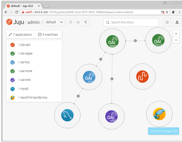
Figure 4: A screen-shot of the Juju Graphical User Interface (GUI), in which virtual elements, i.e., OpenAirInterface (OAI) [28] (LTE Network) and Squid Forward Proxy (App) are instantiated on the MEC-Cloud Infrastructure. This allows the UE attached to an OAI eNB to access the external web-server through a dynamically instantiated Squid forward proxy.
