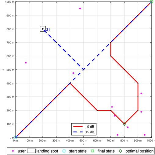
Figure 2. Optimal trajectories for an average cell-edge SNR of 0dB and 15dB with 10 users and one LS.
