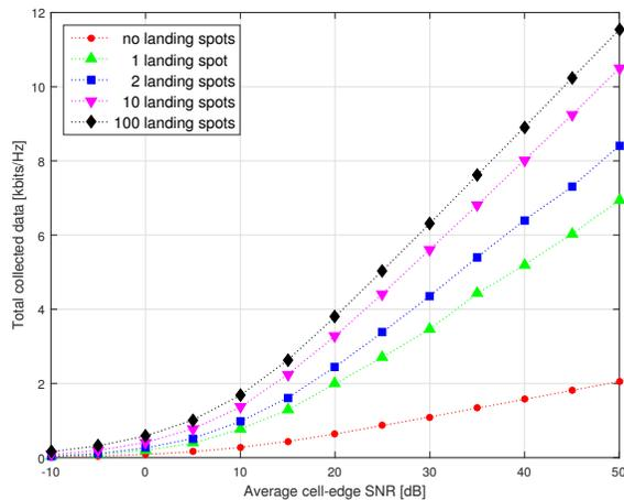
Figure 5. Average throughput for different SNRs and numbers of LSs.
