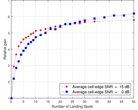
Figure 3. Relative collected data gain for different number of LSs.
