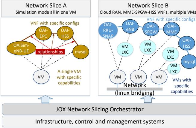
Fig. 1: JOX support for two network slices. In *slice A* the OAI eNodeB and EPC are deployed in a single VM. In *slice B* a cloud-RAN chain using disaggregated RAN is deployed over different VMs.
