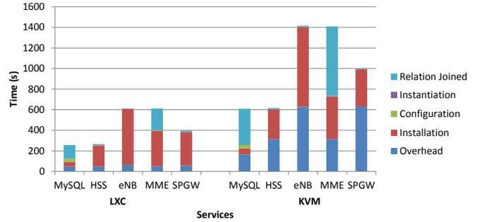
Fig. 10: Deployment time of VNF chains
