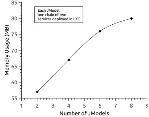
Fig. 9: Effect of increasing the number of slices/models on the memory usage. Every model is a chain of two services (either `mysql-OAI HSS`, or `mysql-apache2`) deployed in LXC.
