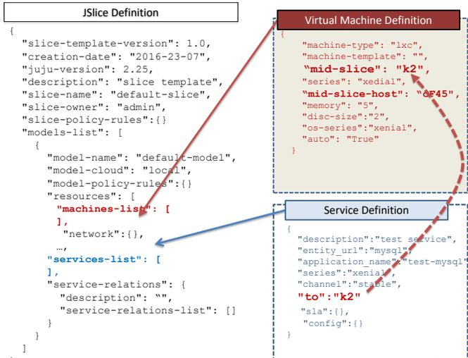
Fig. 5: JOX JSlice definition in JSON representation.
