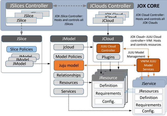
Fig. 3: JOX main components and properties
