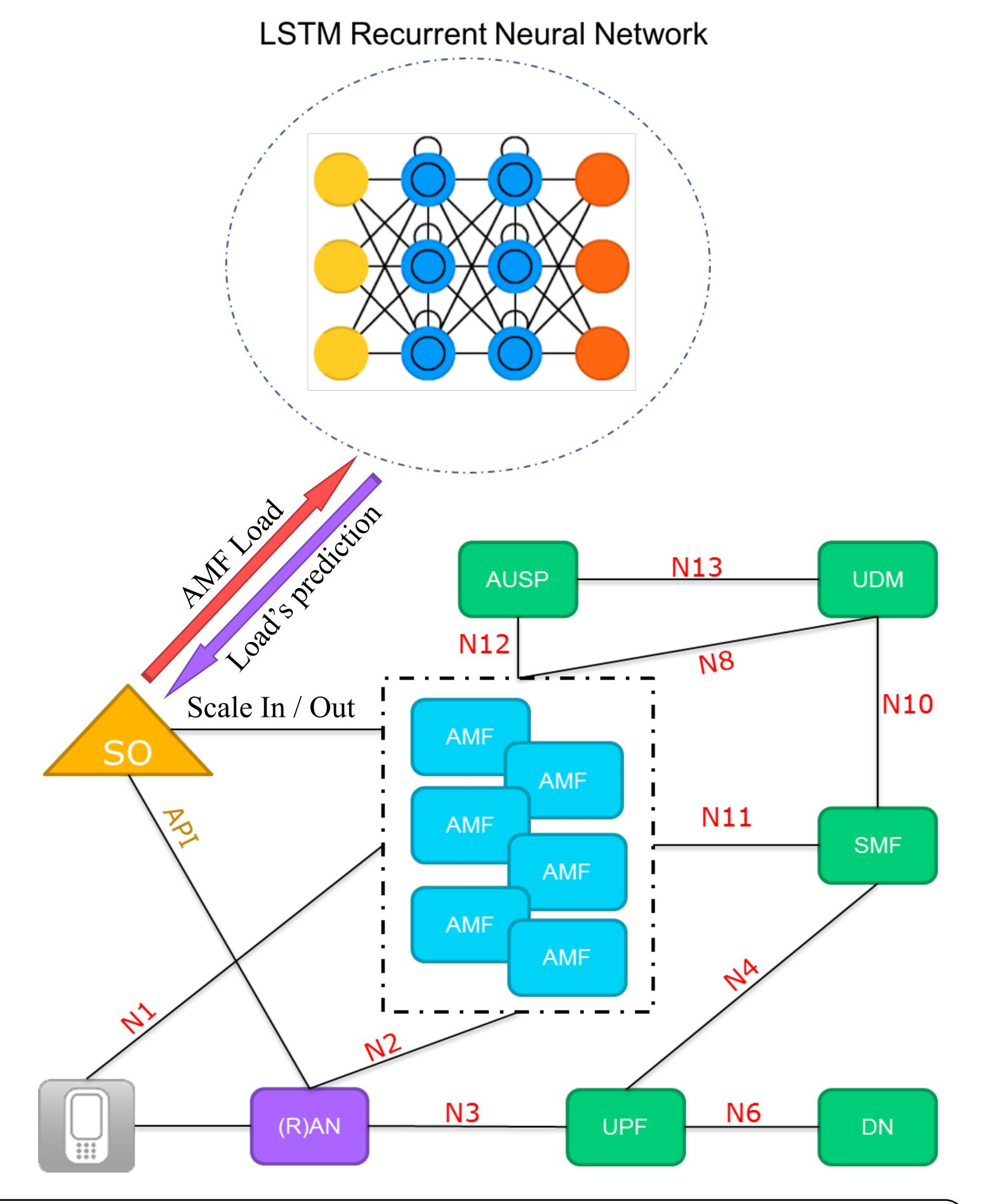
• AMF in the New Generation Core (NGC) [2] architecture is often overloaded due to the fact of being the only access component over the control plane for a huge number of connected devices. This will be particularly exacerbated with regard to the expected number of IoT devices, which will be handled by future mobile networks.
