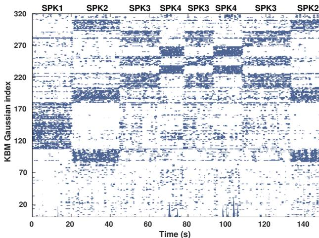
**Fig. 2.** A matrix of BKs from an arbitrary 2.5-minute speech fragment from the ETAPE database. Each column of the matrix is an individual BK with  $N=320$  elements extracted according to the procedure illustrated in Figure 1. Distinguishable BK patterns indicate distinct speakers whereas differences between them indicate speaker change points
