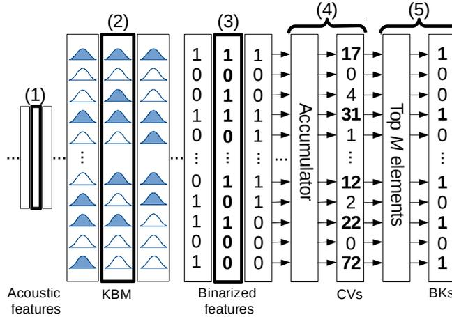
**Fig. 1.** An illustration of the BK extraction procedure based upon the comparison of acoustic features and the KBM
