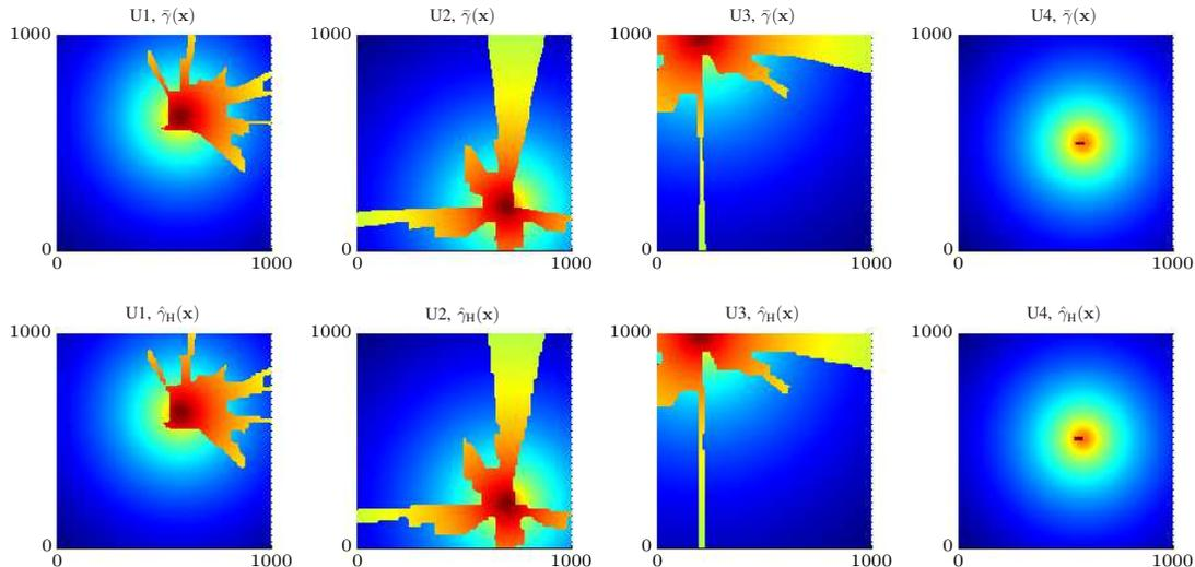
Figure 4. True radio maps  $\bar{\gamma}(\mathbf{x})$  and the reconstructed radio maps  $\hat{\gamma}_H(\mathbf{x})$  for four different user locations. The propagation structures are clearly reconstructed.
