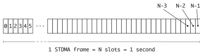
Figure 19 – **STDMA**: channel organization into slots and frames
