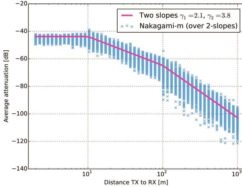
Figure 38 – Dual Slope Propagation with Nakagami-m fading
