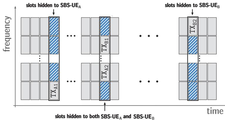
Figure 32 – Half duplex impairment: relative position of TX slots of two SBS-UEs
