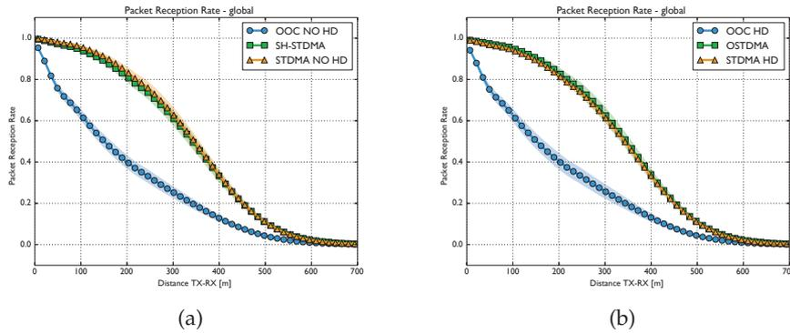
Figure 53 – Packet reception rate versus TX-RX distance
