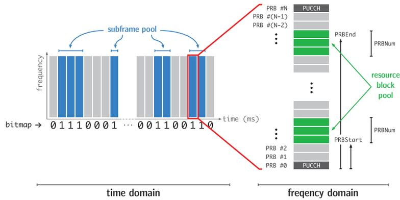
Figure 6 – Resource Allocation in time/frequency domain - Subframe and Resource Block pools
