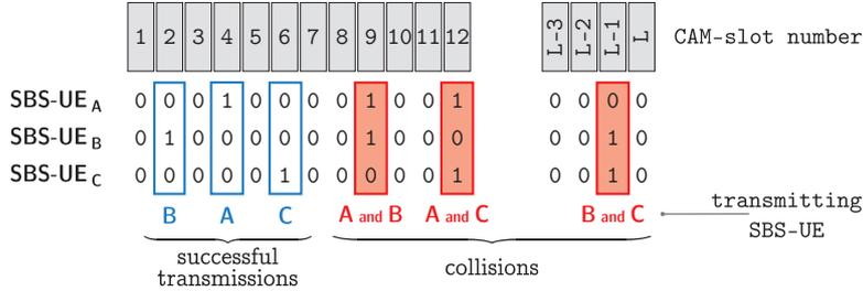
Figure 18 – Distributed Allocation: OOC-based access to slots
