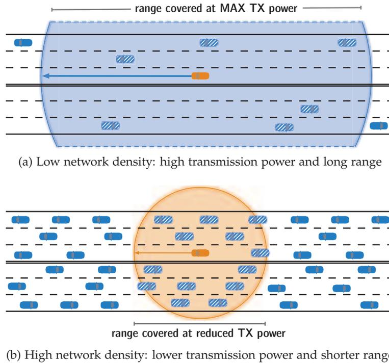
Figure 29 – **Transmission Power Control**: maximum transmission power vs. reduced transmission power
