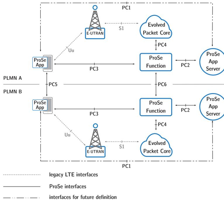
Figure 5 – ProSe architectural extension - adapted from [44, §4.2]
