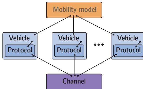
Figure 36 – Static evaluation: simulator block scheme
