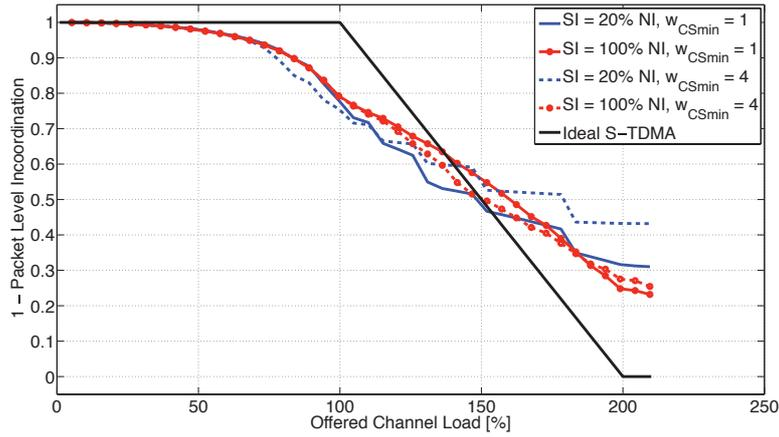
Figure 49 – Packet Level Coordination for  $t_{min} = 3$  and  $t_{max} = 7$
