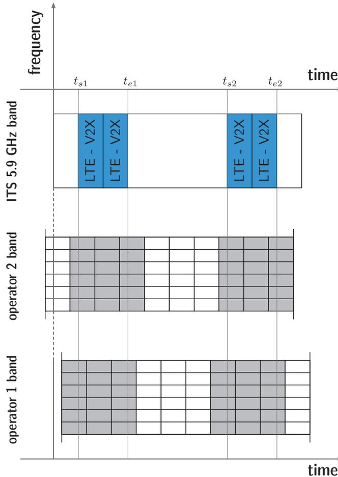
Figure 14 – Outband SBS resource pool: pan operator synchronization. It is shown how the starting time instants of each subframe are not aligned between different operators, and are not aligned to the subframes in the SBS pool. Within the operators’ bands, the subframes that are co-located in time with the subframes belonging to the SBS-pool are highlighted in gray. A transceiver supporting both bands will thus only be able to tune to one of these bands at any give time.
