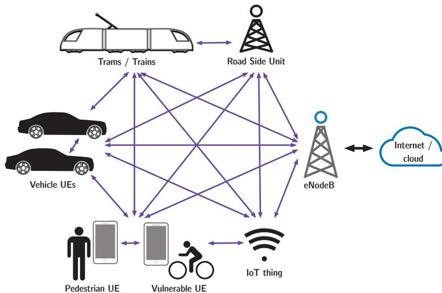
Figure 1 – Connectivity offered by *LTE* plus *LTE-V2X*
