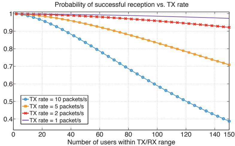
Figure 42 – Tx Rate Adaptation in Unsupervised LTE-D2D
