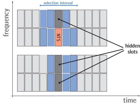
Figure 27 – OSTDMA base principle. Hidden slots, colored in dark gray, are excluded from the candidate set when re-reserving a new NTS
