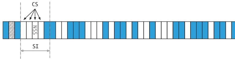
Figure 23 – **STDMA**, network entry phase: **SI** and **candidate set** compilation. *Free* slots are colored in white, *externally allocated* slots are shaded in light blue, and the **NEP** slot is filled with a dash pattern.
