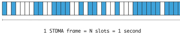
Figure 21 – **STDMA**: initialization phase. *Free* slots are colored in white, whereas **externally allocated** slots are shaded in light blue.
