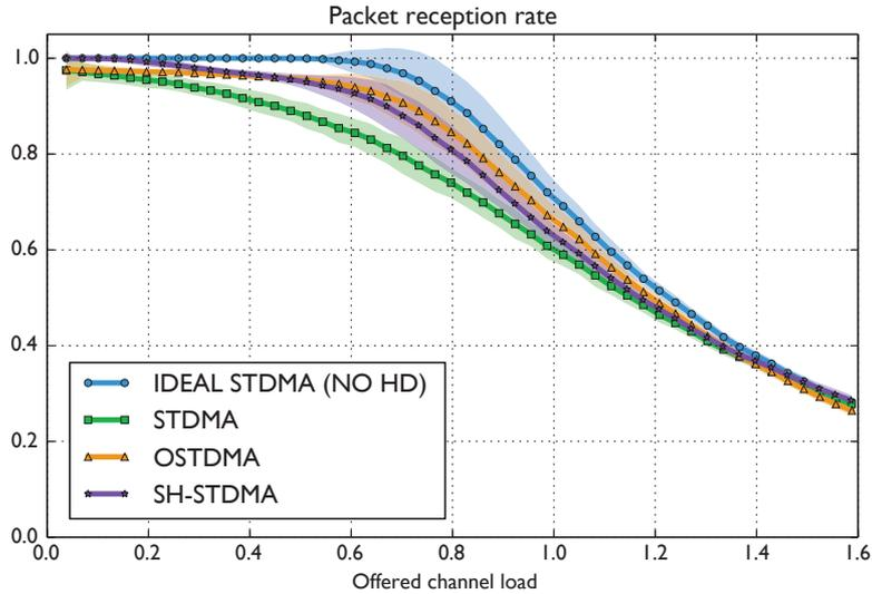
Figure 52 – Protocol extensions: [OSTDMA](#) and [SH-STDMA](#) vs [STDMA](#). The shaded area around the curves represents the 95% confidence interval
