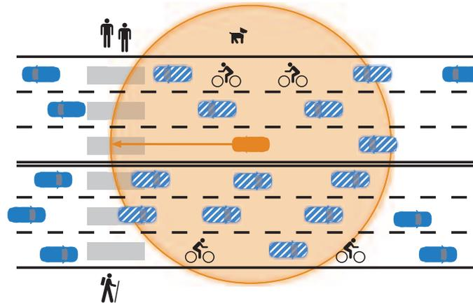
Figure 2 – Single hop broadcast communications
