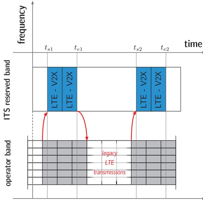
Figure 15 – Distributed Allocation: OOC-based access to slots
