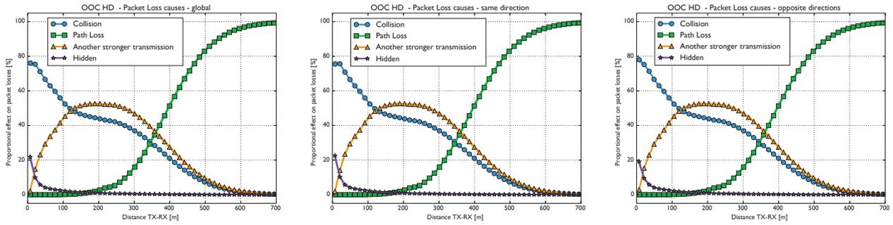
Figure 54 – Causes of packet loss for **OOO** with **HD**, 240 vehicles per km. **Left**: global performance; **center**: only couples of **TX/RX** proceeding in the same direction; **right**: only couples of **TX/RX** proceeding in opposite directions.
