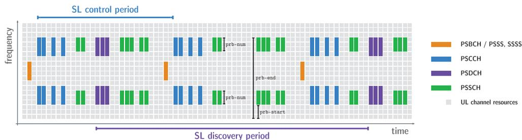
Figure 7 – Example of SL channel structure for transmission mode 2
