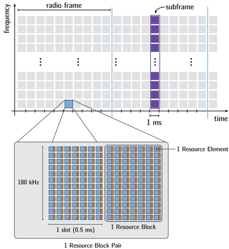
Figure 4 – LTE DL air interface nomenclature
