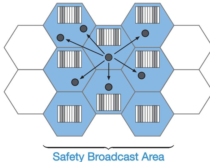
Figure 10 – **Safety Broadcast Area**. It is shown how a **SBS-UE** in the **SBA** can transmit broadcast messages to other **SBS-UEs** within the same area, but in the covering area of different cells. In the cells within the **SBA** a sample radio frame is illustrated, showing a constant set of resources, uniformly allocated all throughout the **SBA**.
