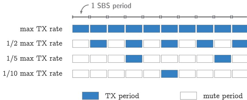
Figure 30 – Transmission Rate Control in OOC
