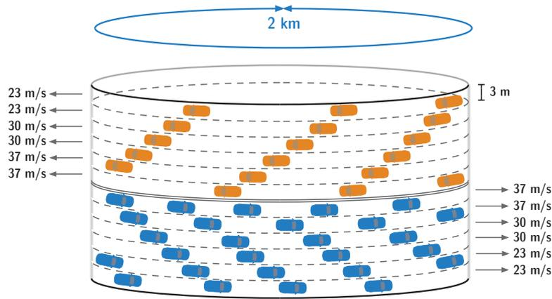
Figure 37 – Dynamic evaluation: highway simulation scenario
