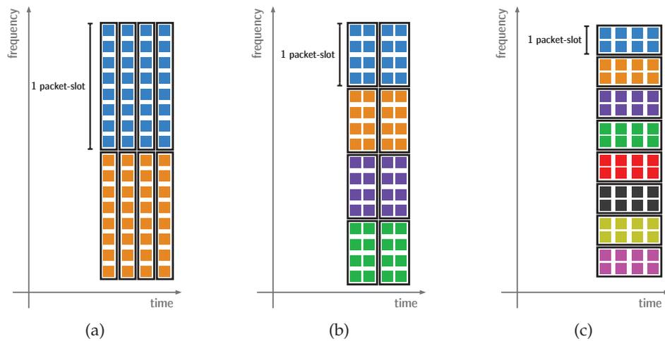
Figure 17 – Partition of the SBS resource pool into packet-slots: time vs. frequency disposition
