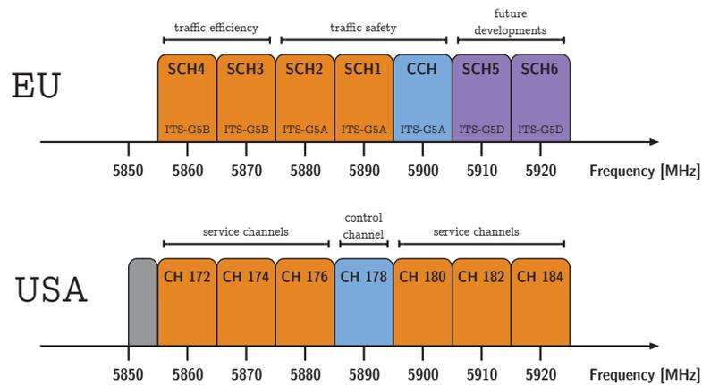
Figure 3 – Frequency allocation plans for ITS-G5 in the EU and DSRC in the USA
