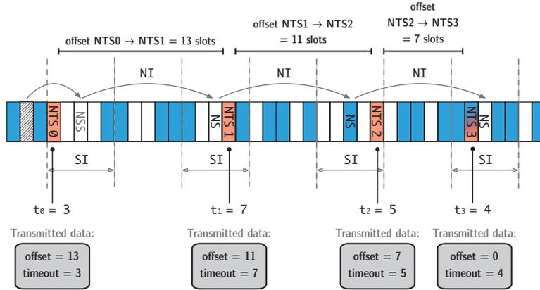
Figure 25 – STDMA, first frame phase: first reservation of the NTSs. Free slots are colored in white, externally allocated slots are shaded in light blue and the NTSs are shaded in red. In this specific example case, NTS #3 is shaded in both red and light blue, as it is a NTS located on a externally allocated slot.
