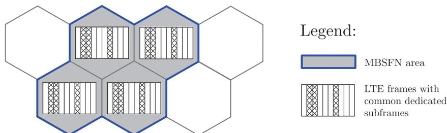
Figure 11 – MBSFN area over multiple cells with common allocated resources.
