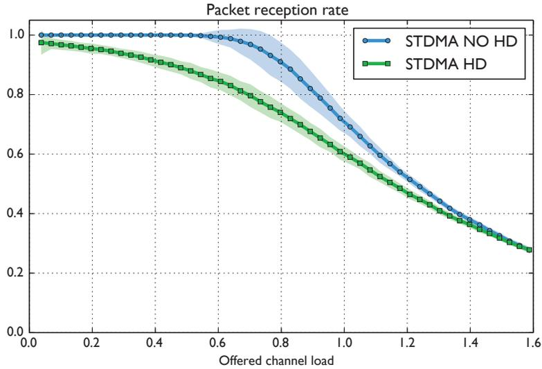
Figure 50 – **STDMA** comparison with and without **HD** impairment. The shaded area around the curves represents the 95% confidence interval
