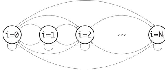
Figure 35 – Markov Chain of the reservation process as seen by the tagged slot. The state variable  $i$  is the number of terminals reusing the tagged slot.
