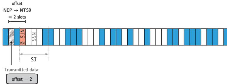
Figure 24 – **STDMA**, network entry phase: **NTS** selection and **NEP** transmission. *Free* slots are colored in white, *externally allocated* slots are shaded in light blue, the **NTS 0** is shaded in red, and the **NEP** slot is filled with a dash pattern.
