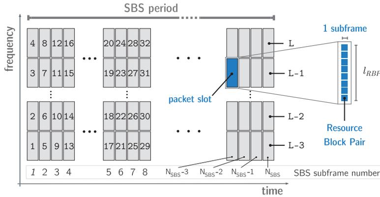
Figure 16 – Partition of the SBS resource pool into packet-slots
