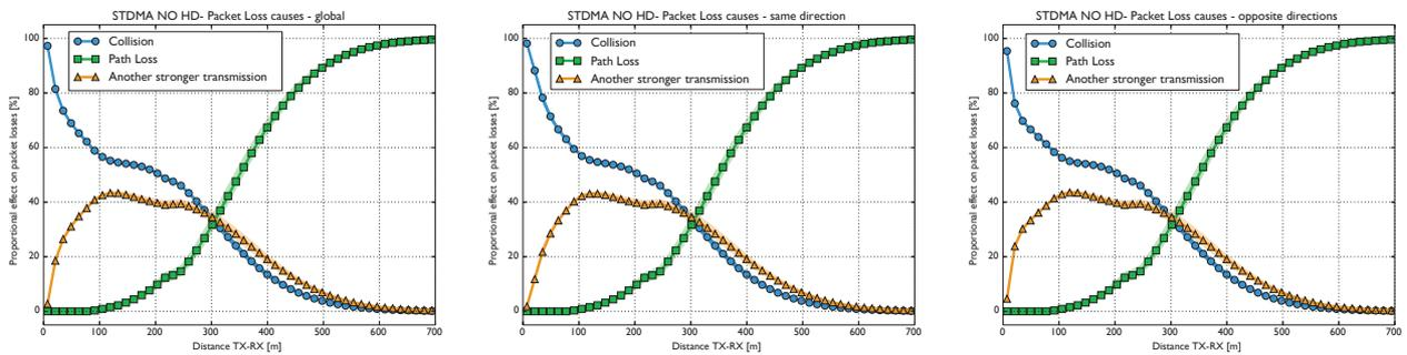
Figure 57 – Causes of packet loss for **STDMA** without **HD**, 240 vehicles per km. **Left:** global performance; **center:** only couples of **TX/RX** proceeding in the same direction; **right:** only couples of **TX/RX** proceeding in opposite directions.
