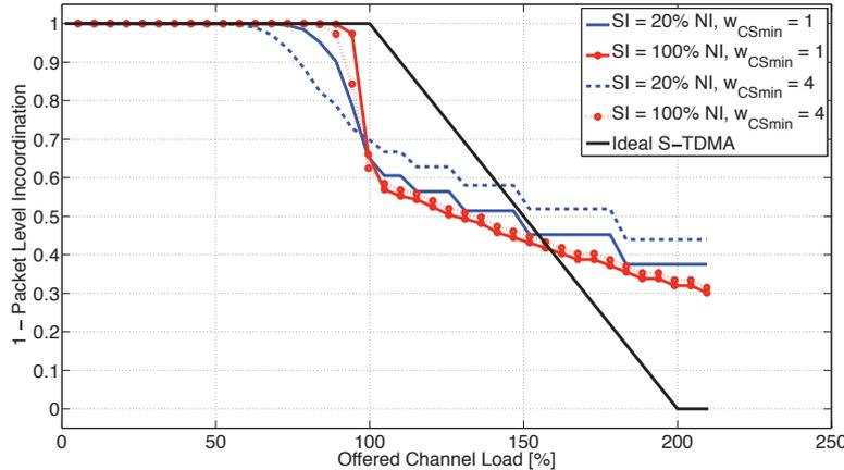
Figure 48 – Packet Level Coordination for  $t_{min} = 1$  and  $t_{max} = 10^5$
