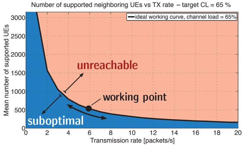
Figure 40 – Transmission rate vs Number of neighboring SBS-UEs for channel load 65%
