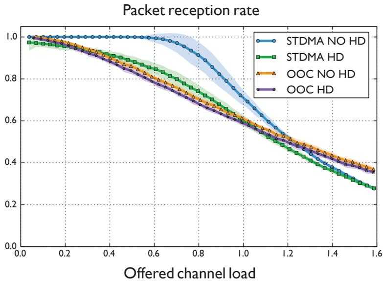
Figure 51 – **STDMA** and **OOC** comparison with and without **HD** impairment. The shaded area around the curves represents the 95% confidence interval
