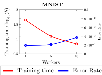
Figure 4: Comparison of training time and error rate for asynchronous DGP-RFF with 1, 5 and 10 workers.
