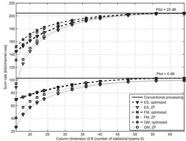
Fig. 1. System sum-rate as a function of the outer precoder dimension for different methods of choosing the outer precoder.
