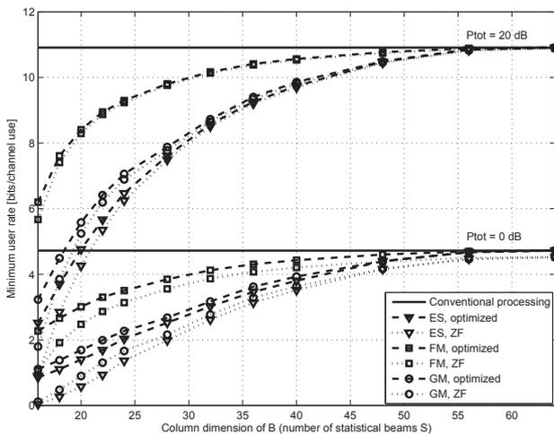
Fig. 2. Minimum user rate as a function of the outer precoder dimension for different methods of choosing the outer precoder.
