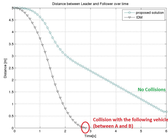
Figure 3: Inter-distance between vehicle A and B , considering an IDM braking strategy.
