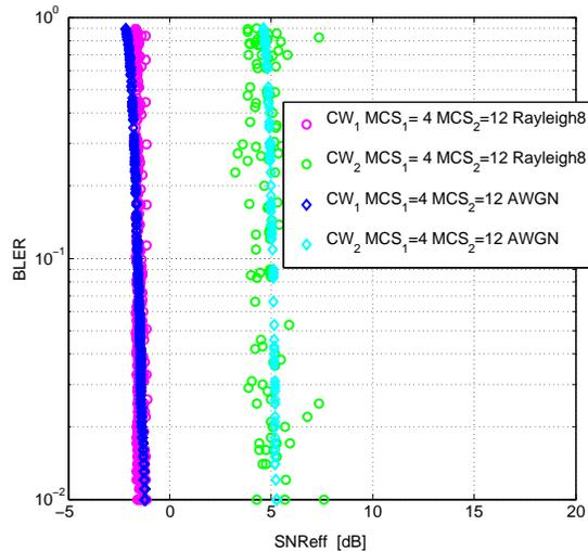
Fig. 4. Performance validation for  $CW_0$  and  $CW_1$  belonging to QPSK and 16QAM respectively. Predicted BLER of TM4 for  $MCS^0 = 4$  and  $MCS^1 = 12$  in 8-tap Rayleigh channel
