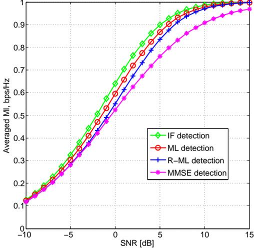
Fig. 1. Average Normalized Sum MI for two CWs belonging to QPSK for 8-tap Rayleigh channel for IF, ML, R-ML PIA and MMSE receivers
