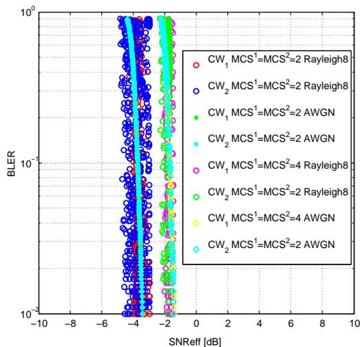
Fig. 2. Performance validation for  $CW_0$  and  $CW_1$  belonging to QPSK. Predicted BLER of TM4 for  $MCS^0, MCS^1 = 2$  and  $MCS^0, MCS^1 = 4$  in 8-tap Rayleigh channel.
