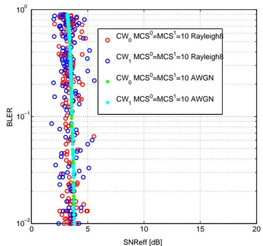
Fig. 3. Performance validation for  $CW_0$  and  $CW_1$  belonging to 16QAM. Predicted BLER of TM4 for  $MCS^0, MCS^1 = 10$  in 8-tap Rayleigh channel.
