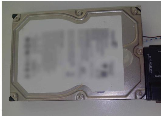
**Figure 3.3:** The disk drive used for experiments. The disk is connected to a SATA (Data+Power) to USB interface (black box on the right) and its serial port is connected to a TTL-serial to USB converter (not shown) via the 3 wires that can be seen on the right.
