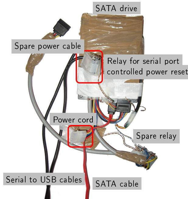
**Figure 4.1:** Custom backdoor development kit. This apparatus was built to reset the drive, allowing easy scripting and automated tasks. One USB to serial cable controls the relay, the second is connected to the serial port of the drive. The SATA cable is connected through a USB-SATA adapter for backdoor development. It is then directly connected to a computer motherboard for the field tests.
