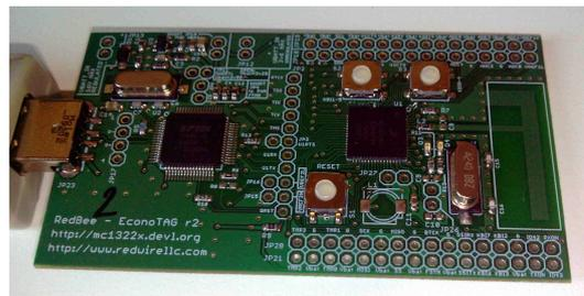
Figure 3.6: The Econotag device. From left to right: the USB connector, serial and JTAG to USB converter (FTDI), Freescale MC13224v controller and the PCB 2.4 GHz antenna.
