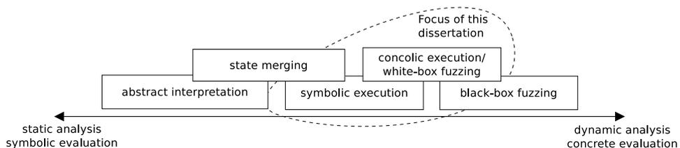
**Figure 2.1:** Relationship of static and dynamic binary analysis methods.
