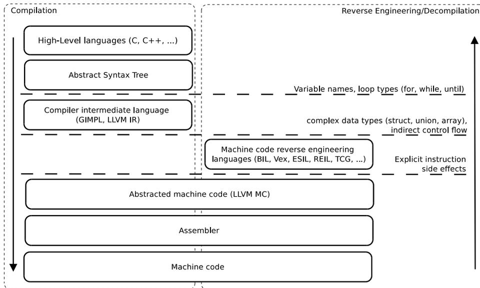
**Figure 2.2:** Positioning of intermediate languages in the compilation/reverse engineering process.
