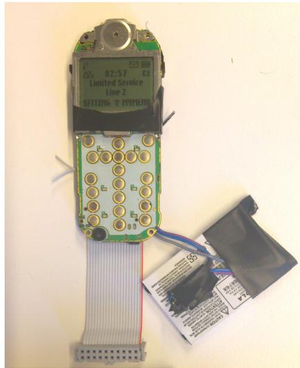
**Figure 3.7:** The Motorola C118. The clip-on battery (on the right) has been wired to the corresponding power pins, while the ribbon cable is connected to the JTAG pads reachable on the back (not shown).
