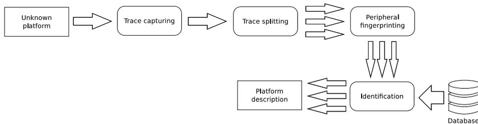
Figure 5.2: Steps for identifying unknown peripherals.
