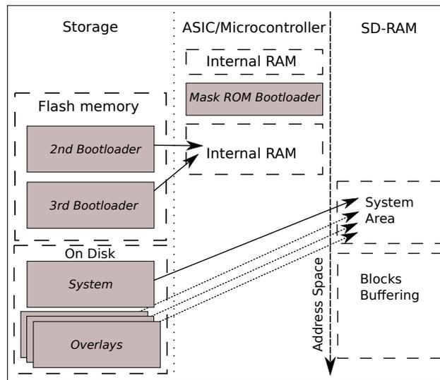
**Figure 4.2:** Overview of a hard drive's architecture.
