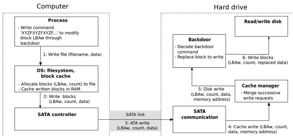
Figure 4.3: Call sequence of a write operation on the hard drive.
