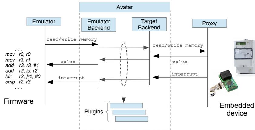
**Figure 3.2:** Avatar architecture and message exchange in full separation mode.
