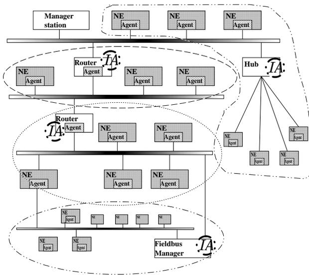
Figure 3: Intelligent Agents spread over a typical management environment.
