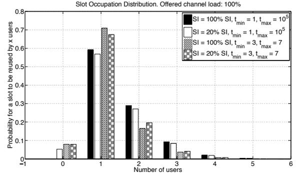
Fig. 5. SOD for OCL = 100%:  $N = 860$ ,  $N_t = 43$ ,  $r = 20$
