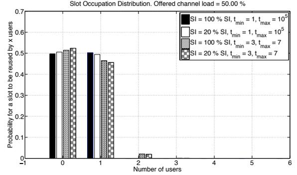
Fig. 4. SOD for OCL = 50%:  $N = 860$ ,  $N_t = 43$ ,  $r = 10$
