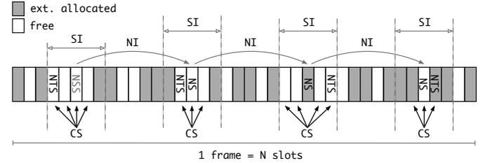
Fig. 1. Slot reservation process: *first frame phase*,  $w_{CSmin} = 3$ . In the SI on the right, two ext. allocated slots had to be included in the CS and a slot reuse is produced (NTS is an externally allocated slot).
