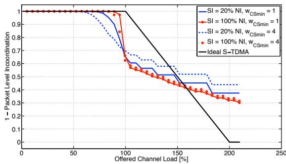
Fig. 6. Packet Level Coordination for  $t_{min} = 1$  and  $t_{max} = 10^5$
