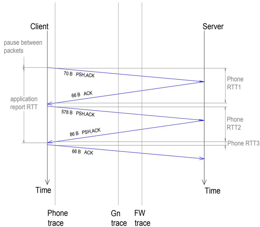
**Fig. 2.** Different RTTs calculated in the phone trace, for a sequence of packets corresponding to one application generated packet.
