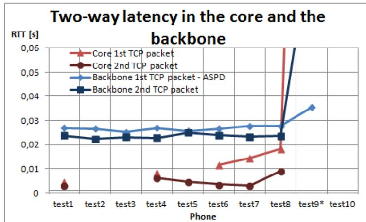
**Fig. 6.** Two-way latency in the core network and the backbone
