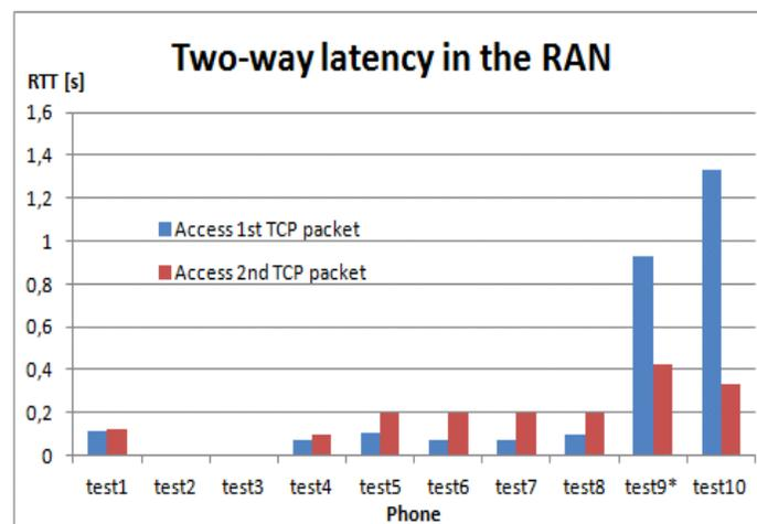
**Fig. 5.** Two-way latency in the RAN (Radio Access Network).
