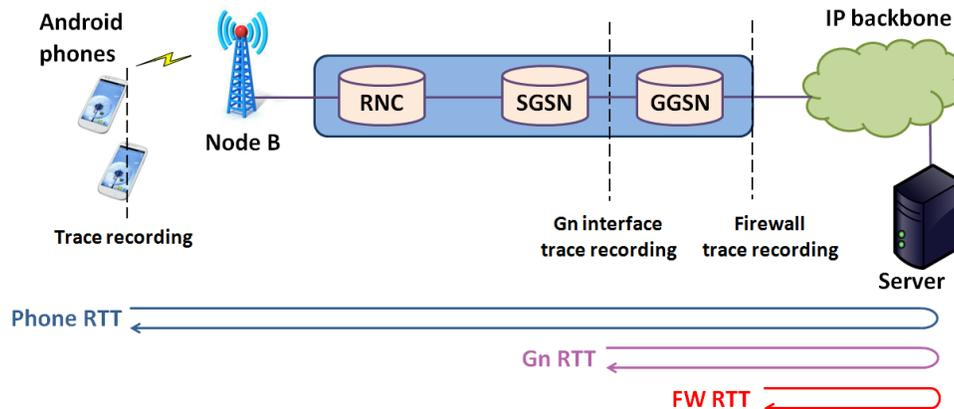
**Fig. 1.** Measurement setup.
