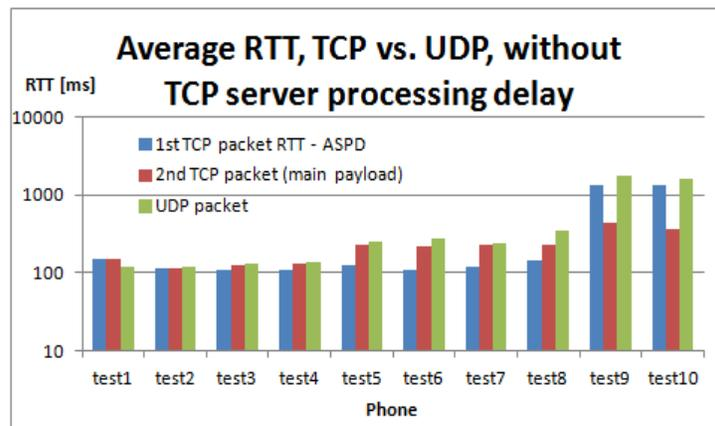
**Fig. 3.** TCP vs. UDP latency: average recorded RTTs, with average server processing delay subtracted from the 1<sup>st</sup> TCP packet RTT, logarithmic scale.
