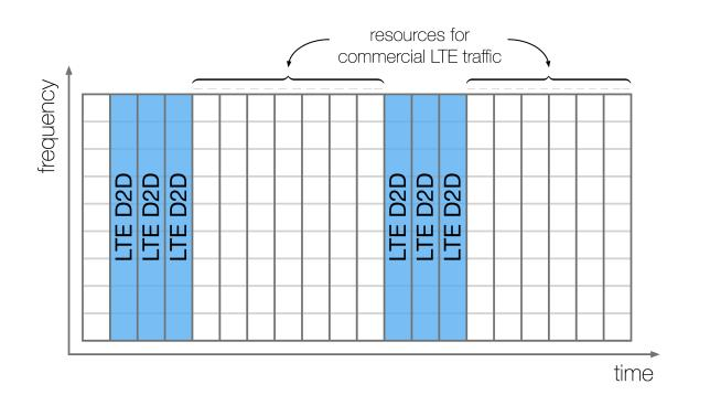
**Dedicated band:** D2D subframes allocated in reserved band (5.9 GHz). Allows time sharing with DSRC
