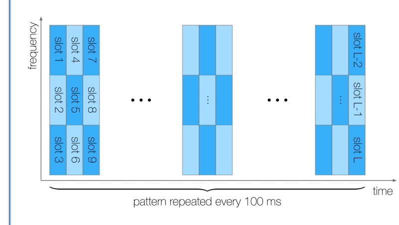
Resource blocks belonging to the subframes dedicated to LTE D2D broadcast are collected into slots the size of a CAM packet
