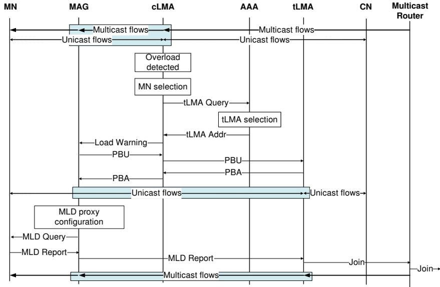
Figure 1: IP Multicast in the reactive-MN approach.
