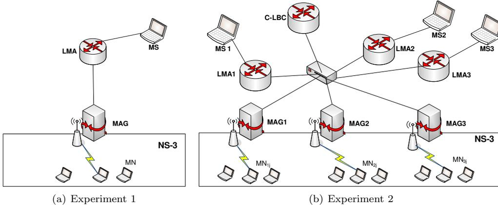
Figure 6: Evaluation Testbeds.
