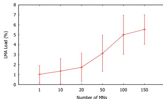
Figure 7: Load versus number of MNs (scenario 1, experiment 1).
