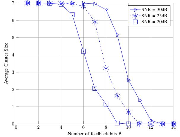
Fig. 2: Cluster size as a function of  $B$  in a 7 cell equal pathloss network.
