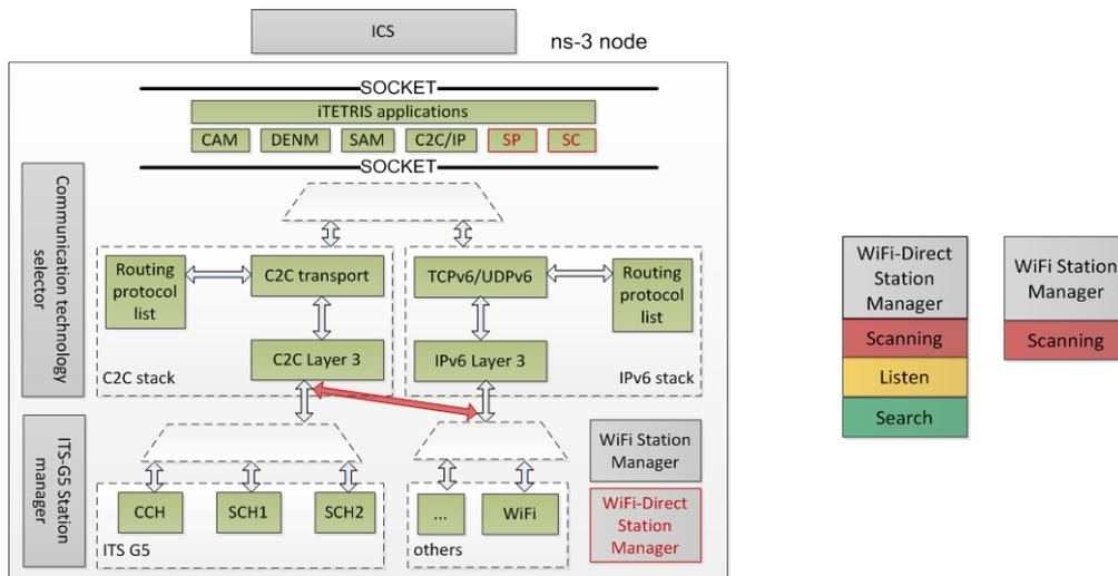
Figure 6 ns-3 extensions for COLOMBO (in red) - WiFi-Direct support, Service Provider (SP), Service Consumer (SC) as well as C2C Stack on WiFi-Direct. The WiFi-Direct Station Manager implements two new WiFi-Direct P2P Discovery (Listen/Search phases)
