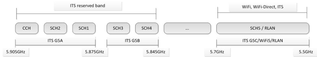
Figure 5 Spectrum Allocation at 5GHz - ITS G5, WiFi 5, and WiFi-Direct
