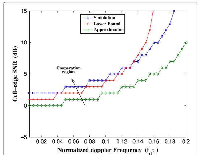
**Figure 7** Cooperation region: cell edge SNR vs. Doppler frequency. With only a feedback delay of 1 symbol time.
