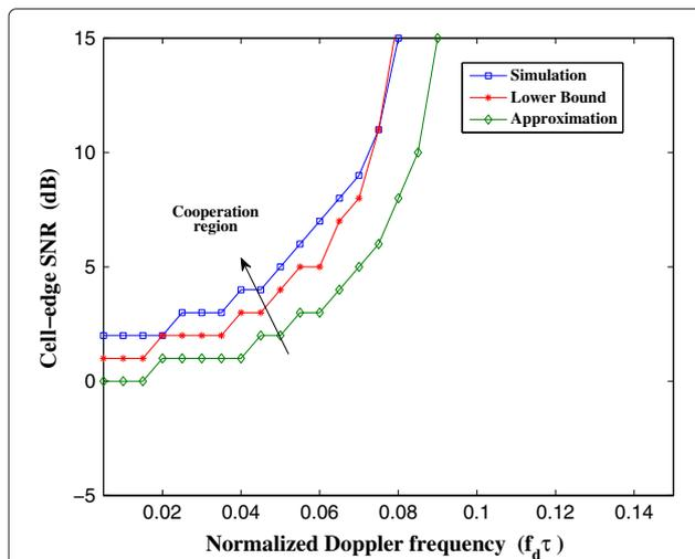
**Figure 6** Cooperation region: cell edge SNR vs. Doppler frequency. With a feedback delay and back-haul delay of 1 symbol time each.
