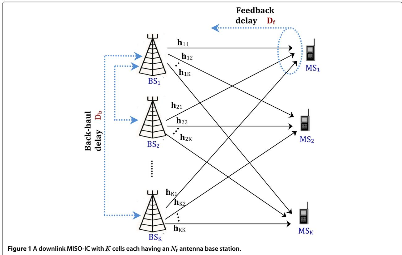
Figure 1 A downlink MISO-IC with  $K$  cells each having an  $N_t$  antenna base station.
