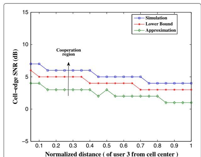
**Figure 8** Cooperation region: cell edge SNR vs. normalized distance. With a Doppler frequency of 0.05, and a feedback delay and back-haul delay of 1 symbol time each.
