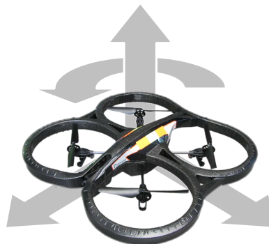
Figure 1: AR.Drone 2.0 quadcopter: Its 4 degrees of freedom during flight are indicated by arrows.
