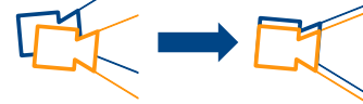
Figure 8: Video stabilization for moving object masking, used while hovering before or after a height change for dense 3D perception
