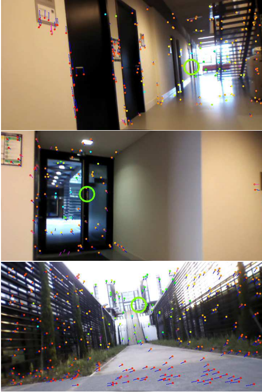
Figure 5: Sparse 3D reconstruction results: Blue/purple lines show optical flow vectors consistent/conflicting with the quadcopter’s motion. The points’ color indicates their longitudinal distance – red stands for 1 m and below, cyan for 10 m and above. A larger green circle marks the target flight direction.
