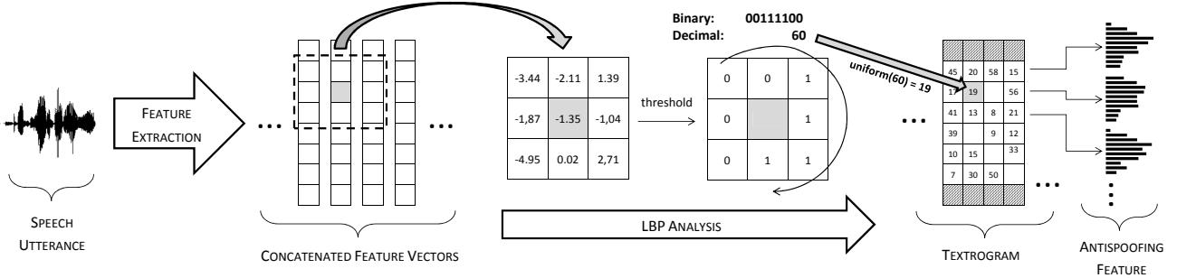
Figure 1: Application of uniform LBP analysis to obtain a textrogram from a matrix formed from the concatenation of conventional feature vectors. Non-uniform patterns (blank cells in textrogram) are discarded and the resulting feature used for spoofing detection is formed from the concatenation of normalised histograms of the remaining uniform codes in each row.
