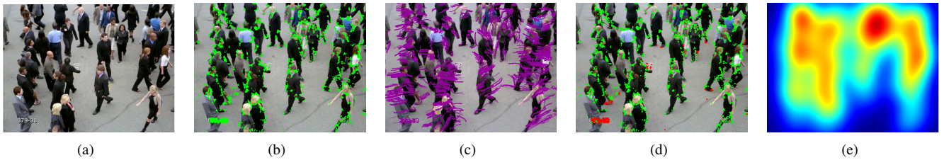
Fig. 1. Illustration of the proposed crowd density map estimation using FAST as local features: (a) Exemplary frame, (b) Local feature points by FAST algorithm, (c) Feature tracks, (d) Distinction of moving (green) and static (red) features - red features at the lower left corner are due to text overlay in the video, (e) Estimated crowd density map
