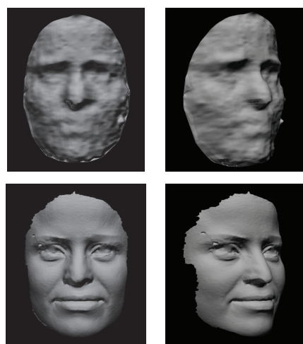
Illustration of the low quality face data obtained by Kinect (upper row) and the high quality face data obtained by Minolta (lower row) of the same person.
