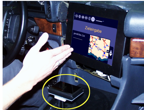
Figure 40: Gesture control of infotainment menus [Geiger, 2003]
