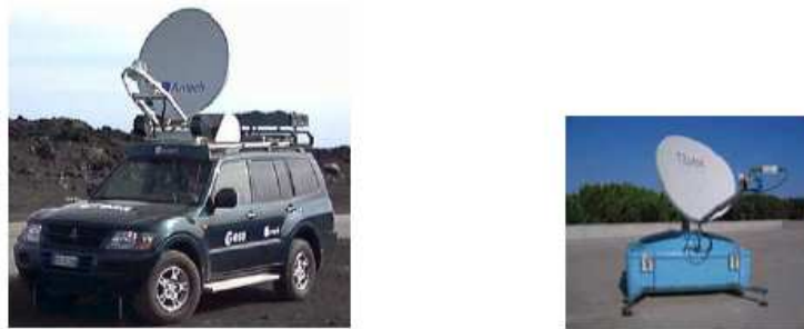
Figure 6.10: ESA Pajero and Temix EasyFlySat terminal.
