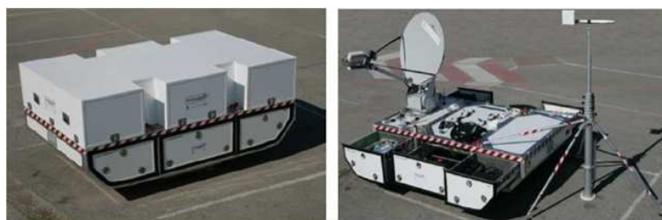
Figure 6.16: Emergesat container before and after installation.
