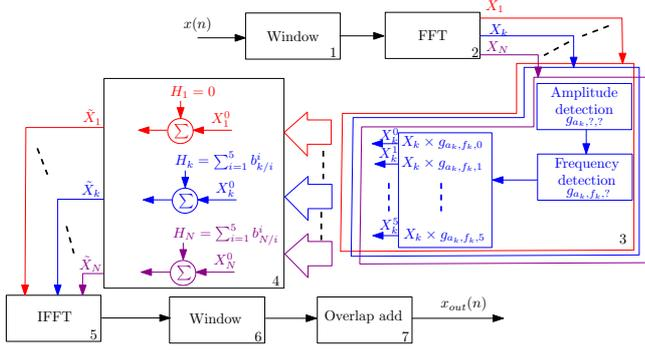
Fig. 2. The frequency domain model. The input signal is windowed and transformed into the frequency domain where the harmonic distortions are introduced according to the amplitude-dependent matrices described in Section II.
