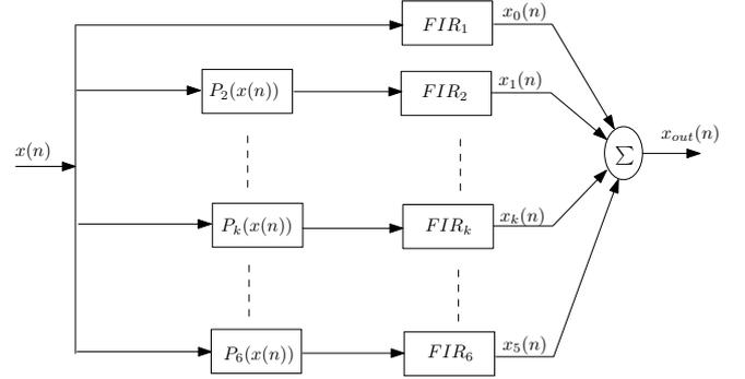
Fig. 3. I/O system of the polynomial model, the signal is processed in each stage to obtain a harmonic order distortion
