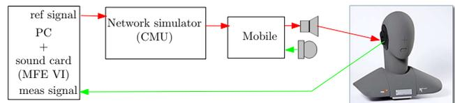
Fig. 1. An illustration of system setup. Reference signals are sent to a mobile terminal via a network simulator and are recorded with a high-quality microphone at the ear of a mannequin.
