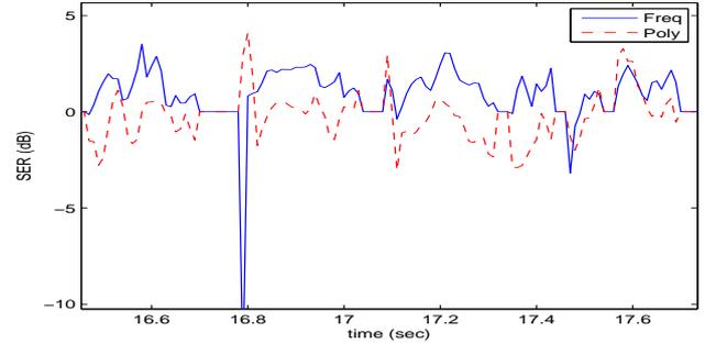
Fig. 4. Signal-to-estimate ratio (SER) against time for the two loudspeaker models. The frequency domain distortion model underestimates the real output whereas the polynomial model overestimates the real output.
