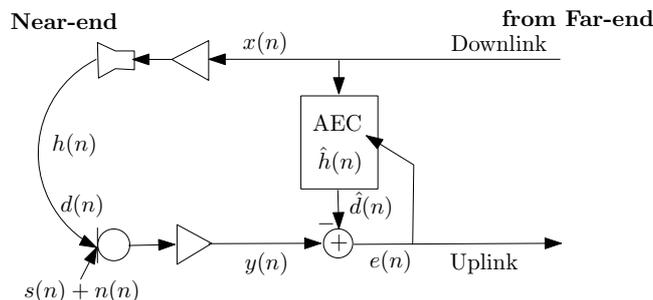
Figure 1: System/echo model illustrating the acoustical coupling between the loudspeaker and microphone and a general approach to adaptive AEC.
