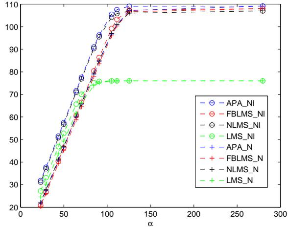
Figure 2: Maximum  $ERLE$  (in dB) achieved after convergence as a function of  $SNR/SNeR$  (also in dB). Here the  $SNR$  or  $SNeR$  corresponds to added noise or to non-linear echo as indicated. Profiles are illustrated for both perturbations and for each of the four approaches to AEC. APA, FBLMS and NLMS are all configured to give equivalent performance under linear echo conditions.
