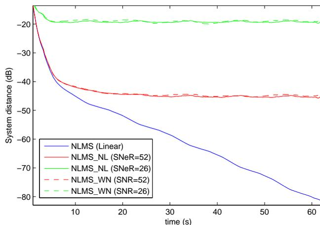
Figure 4: Plots of system distance (in dB) against time (in seconds) for the NLMS algorithm. Profiles are illustrated for linear echo and also for linear echo with either non-linear echo or added noise at two different levels.
