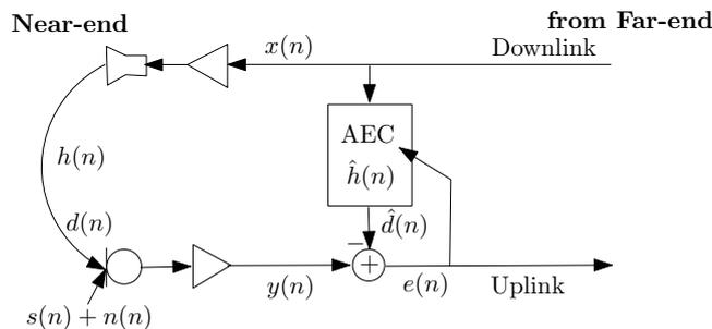
Figure 1: System/echo model illustrating the acoustical coupling between the loudspeaker and microphone and a general approach to adaptive AEC.
