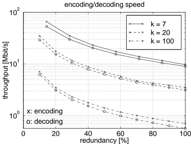
Figure 1: Coder and decoder throughput in Mbits/s with respect to the percentage of redundancy  $h/k \cdot 100\%$  and the TG size  $k$ .
