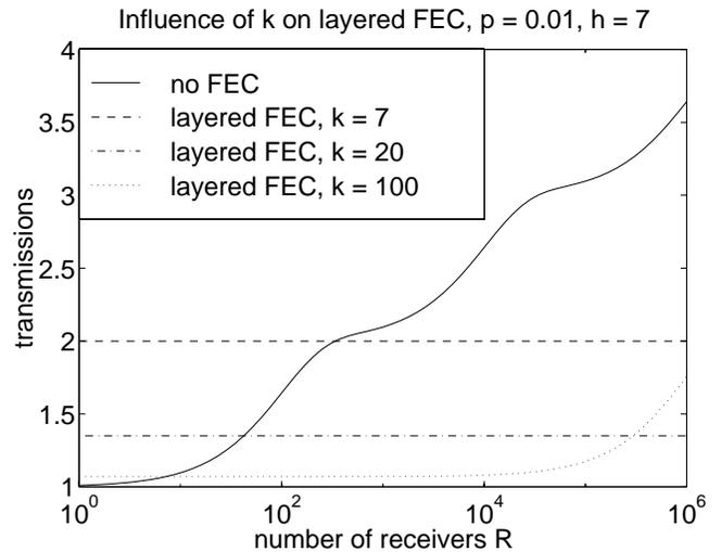
Figure 4: Non FEC versus layered FEC with  $h = 7$  parity packets for different TG sizes  $k = 7, 20, 100$  and loss probability  $p = 10^{-2}$ .
