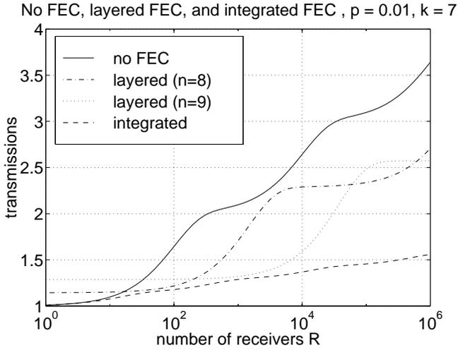
Figure 5: Comparison of non FEC, layered FEC ( $n = 8, 9$ ), and integrated FEC ( $n = \infty$ ) for  $k = 7$  and  $p = 10^{-2}$ .
