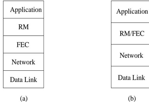
Figure 2: (a) Layered FEC. (b) Integrated FEC.
