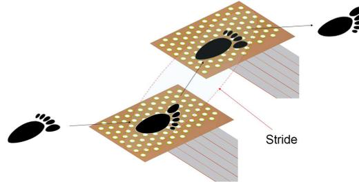
**Fig. 7** Spatial distribution of the piezoelectric sensors.
