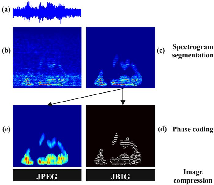
**Fig. 3.** Figure illustrating a 4 digit speech signal degraded by car noise to 0dB undergoing spectrogram segmentation coding
