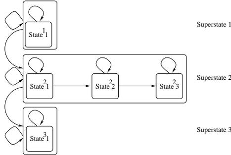
**Fig. 2.** A pseudo two-dimensional extension of the 1DHMM shown in Figure 1.
