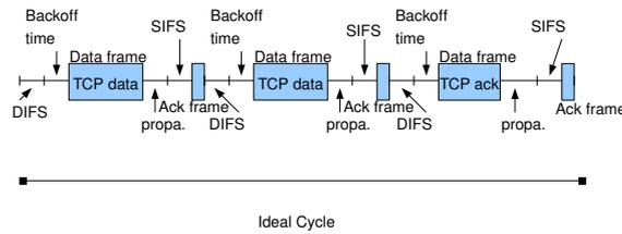
Figure 9: Ideal cycle of data exchanges on the wireless channel for download traffic only scenario
