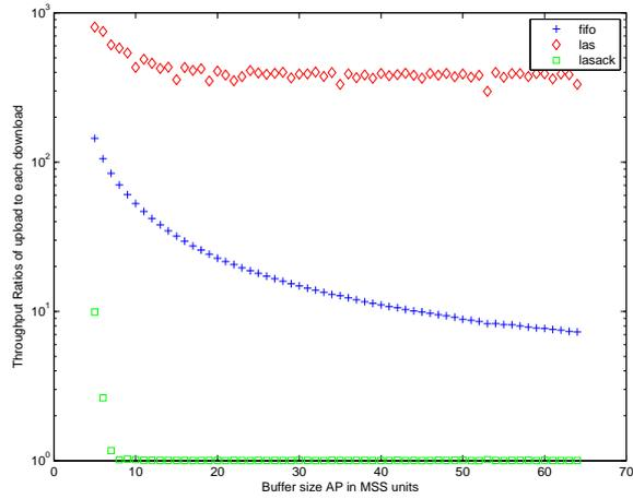
Figure 3: Ratio of upload to download throughputs w.r.t. buffer size at the Access point
