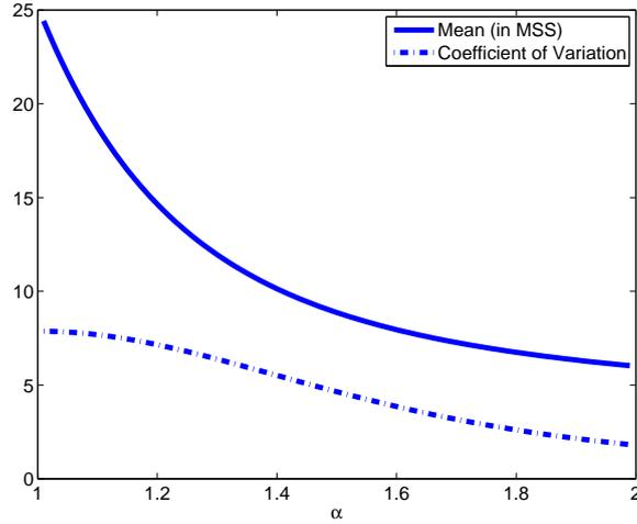
Figure 8: CoV and mean value for a Bounded Pareto distribution for  $k = 4.5$  kbytes,  $P = 20$  Mbytes
