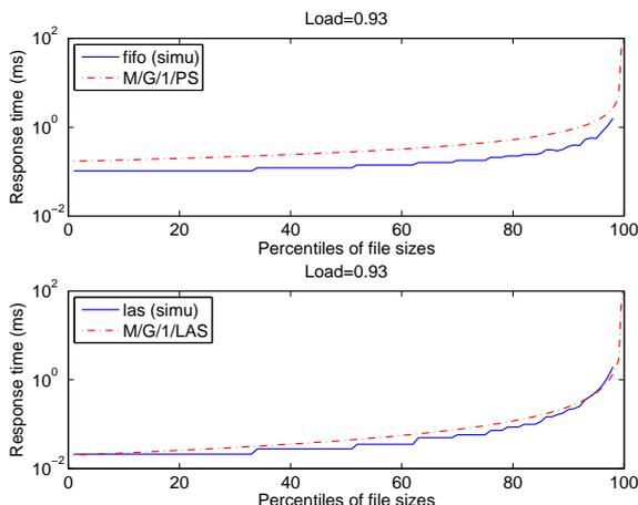
Figure 18: Response time at the access point for an offered load of 3 Mbits/s. Bounded Pareto distribution - CoV=5.5
