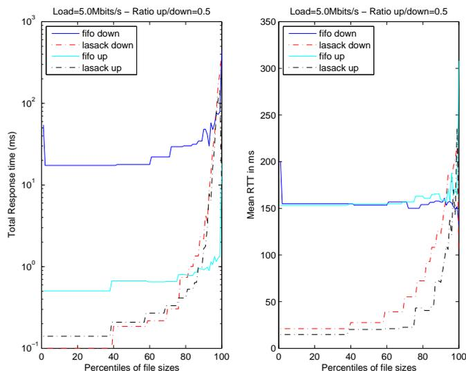
Figure 20: LASACK vs FIFO for a total input load of 5 Mbits/s
