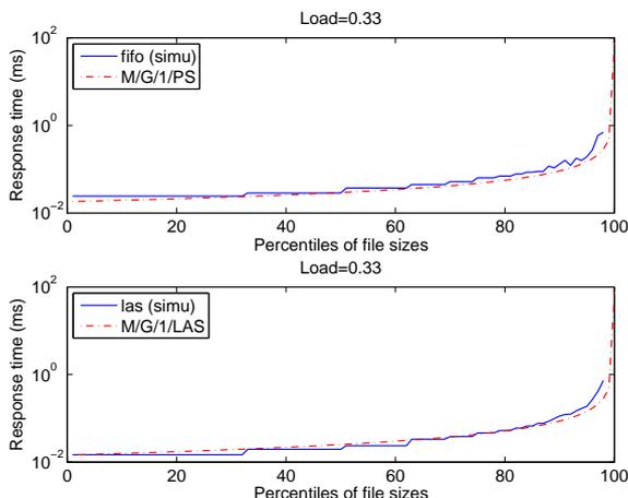
Figure 16: Response time at the access point for an offered load of 1 Mbits/s. Bounded Pareto distribution - CoV=5.5
