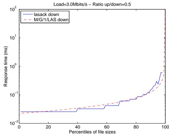
Figure 21: Response time of download traffic at the access point for an offered load of 3 Mbits/s
