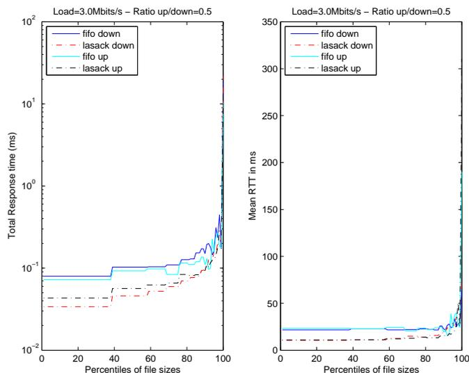
Figure 19: LASACK vs FIFO for a total input load of 3 Mbits/s
