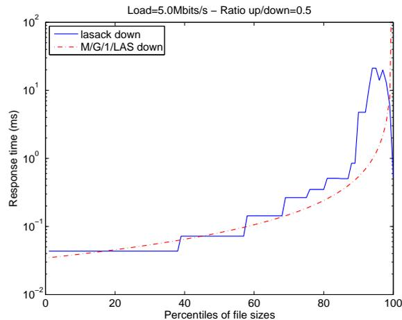
Figure 22: Response time of download traffic at the access point for an offered load of 5 Mbits/s
