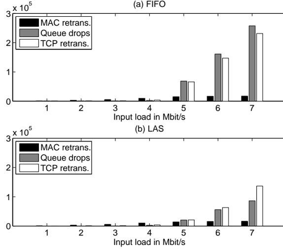
Figure 15: Impact of workload increase on the different layers of the protocol stack
