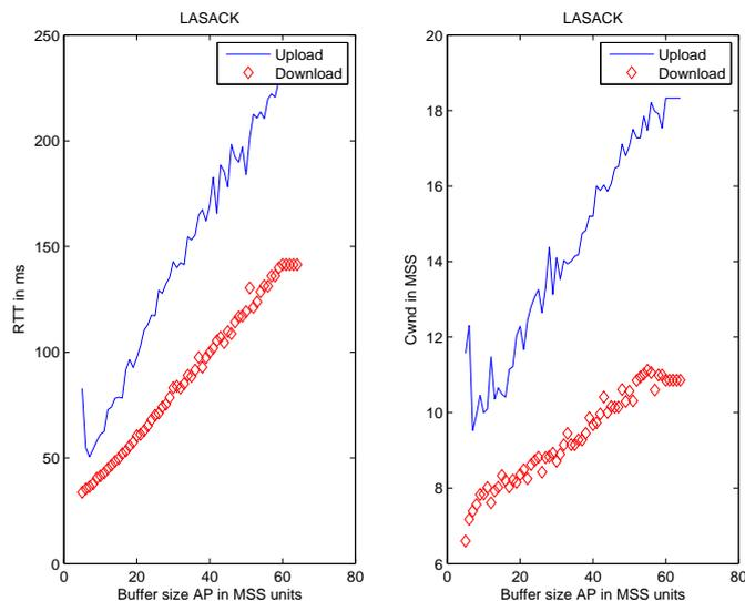
Figure 6: RTTs (left) and Cwnd(right) w.r.t. buffer size at the Access point, under LASACK
