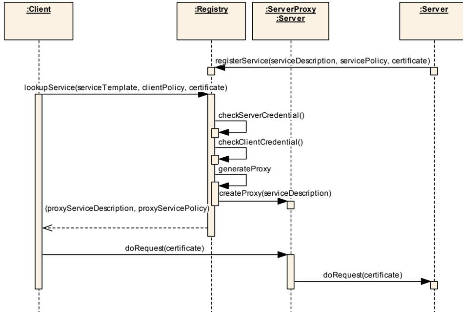
Fig. 6. Secure Service Discovery: the Backup Service
