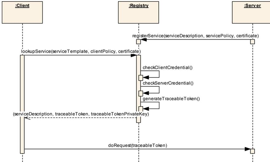
Fig. 4. Secure Service Discovery: the Photo Printing Service
