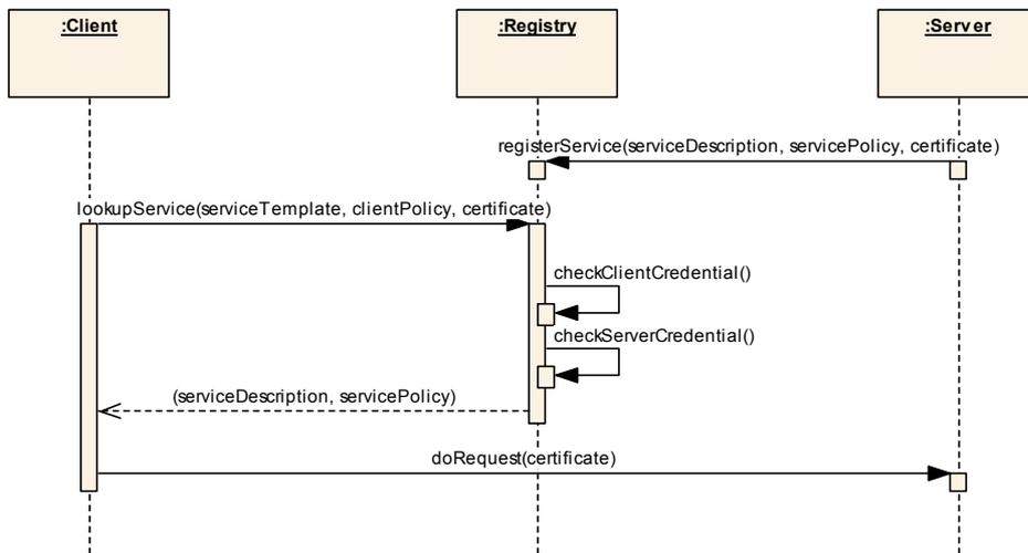
Fig. 5. Secure Service Discovery: the File Sharing Service
