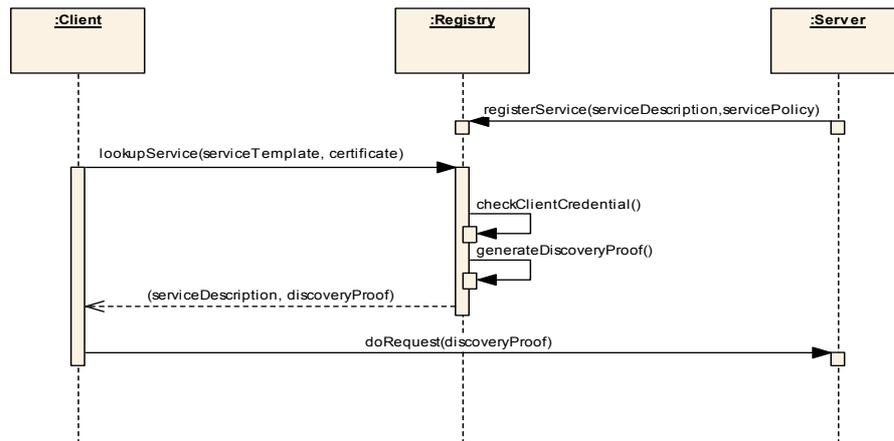
Fig. 3. Secure Service Discovery: the Color Printing Service
