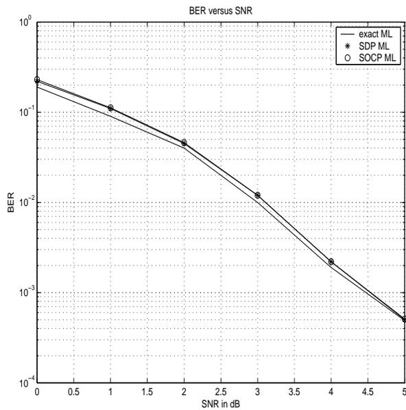
**Fig. 2.** Av. BER for  $N=2$ ,  $M=2$  vs  $SNR(dB)$ .
